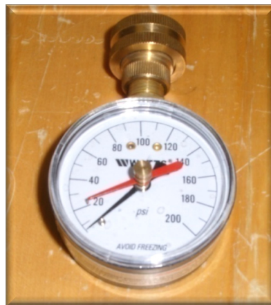
Figure 15: Input Line Pressure Meter (psi)
